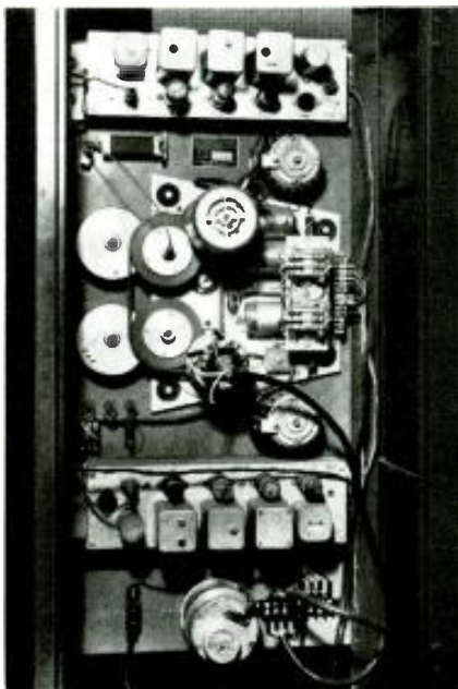
INTERLOCK MOTOR mounting on the 35-mm projector.
